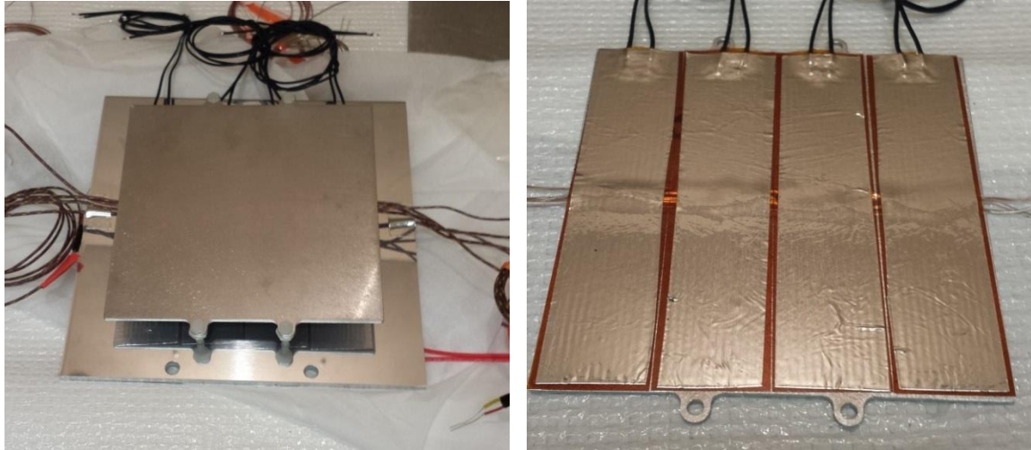
Figure 5.1. Test article, front and back. Primary test surface has 4 independently controlled 1"x4" (2.54 x 10.16 cm) heaters (right), aluminum tape is included to reduce potential for heater-damaging hot spots.
